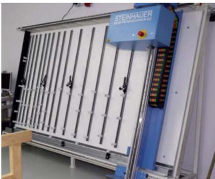
Drilling machine for mounting plates
